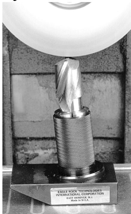
Shellmill arbors on page 5-6 are required for grinding Shellmills.
