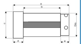
Type II Bushette Obstructed "Through Hole" For R8 and 2MT Collets
